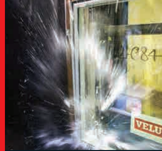
The skylights were hit at their weakest points - the corners
