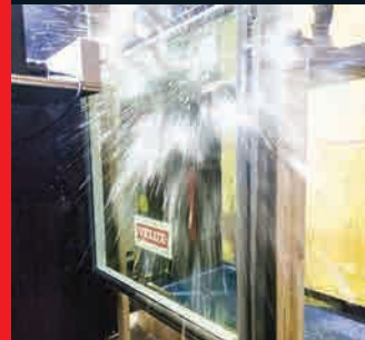
Each skylight was hit four times with 50 mm hailstones at 135 kph and four times with 72 mm hailstones at 150 kph+
