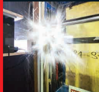
At the end of the test there was no damage at all on any of the three VELUX skylights
